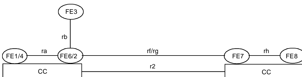
Figure 6: Example relationship between models for ANF-ISIIC and basic call in the case of called user hSwMI being SwMI A
